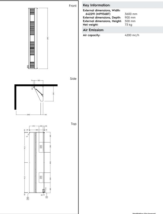
Ventilation Equipment 430 S/S Wall Hood+Filters 3600X900mm
